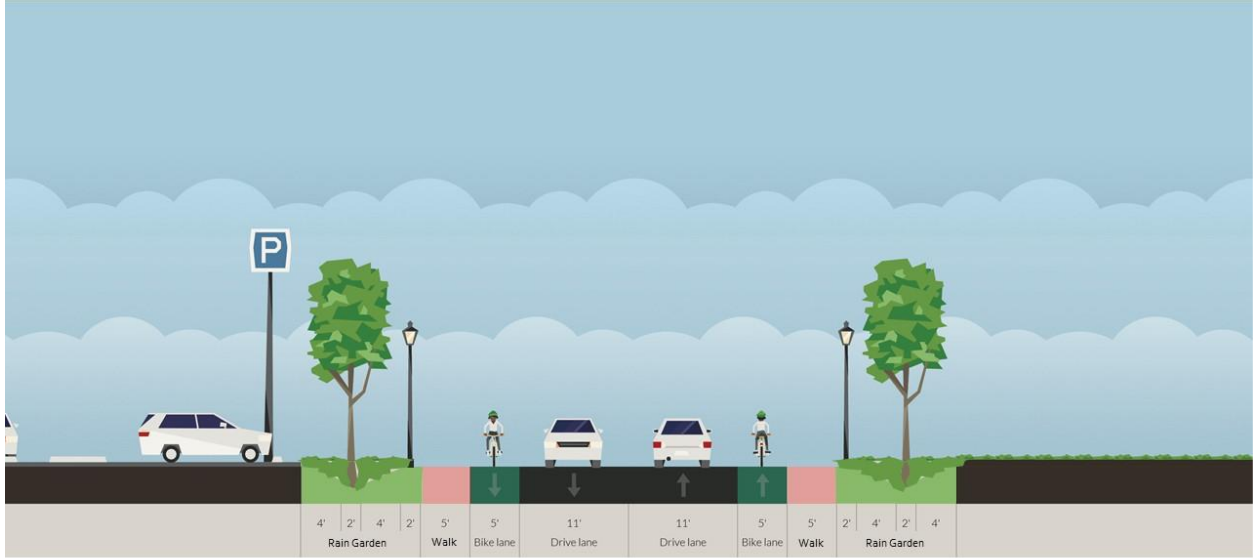
N. Palafox Street Combination Bike-Ped Lane with Rain Gardens
