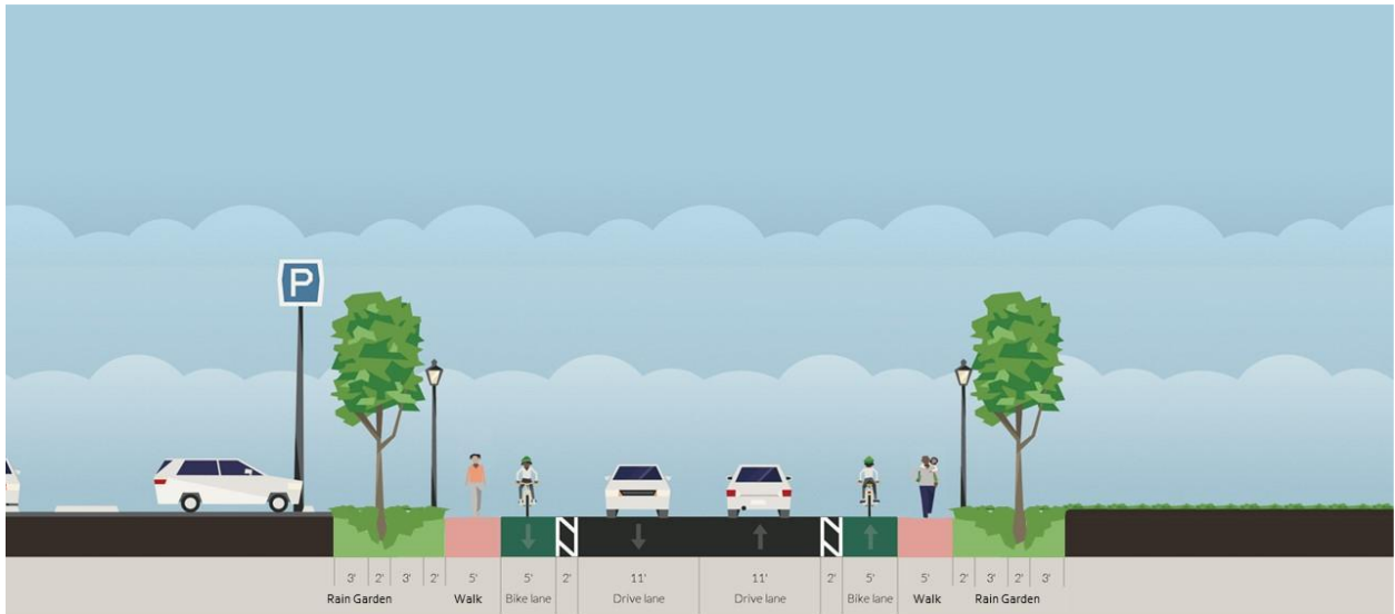
N. Palafox Street Combination Buffered Bike-Ped Lanes with Rain Gardens
