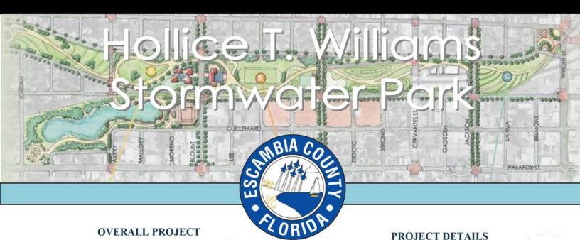
This project will construct a dual use stormwater and recreational-use basin under the Interstate 110 corridor. The project will aid the City of Pensacola in collecting, treating and routing 1.3 miles of stormwater that runs off elevated lengths of Interstate 110 near its southern terminus, providing relief to diverse historical neighborhoods in flood prone areas near Hollice T. Williams Park.
