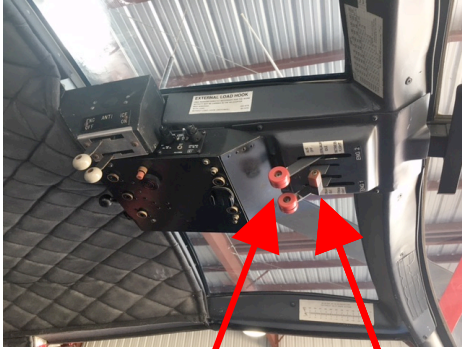
Overhead throttle x2 – aft to first detent. Depress two inner safetys, then fully aft.
