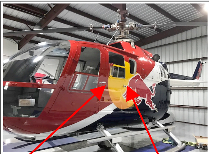
Front door handle – swing down to open
