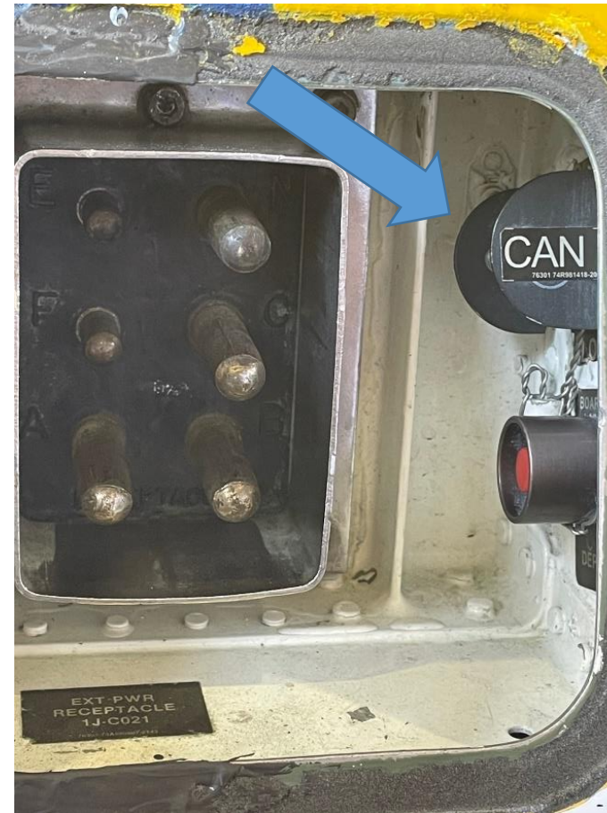
Canopy Toggle Switch (Up for Up)
